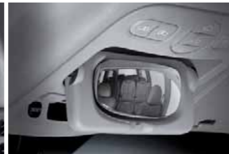
The conversation mirror allows the driver to see everything that's going on in the back at a glance.
