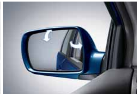
Electrically adjustable door mirrors on all models with heated mirrors on high grade models and electrically folding (high grade).
